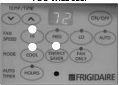
Note: In this mode, when the compressor shuts off, the fan will continue to run for another 3 minutes, then shut off until cooling is needed, as sensed by the room temperature control. During this time, it may come on for 3 minutes to sense whether cooling is needed, then it will go off for 15 minutes. It will continue doing this to sample the room air for as long as necessary.
